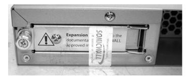
Figure 4: Tamper Seal #3 - Expansion Bay
