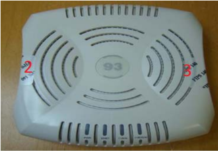
Figure 10 - Aruba AP-93 TEL placement top view
