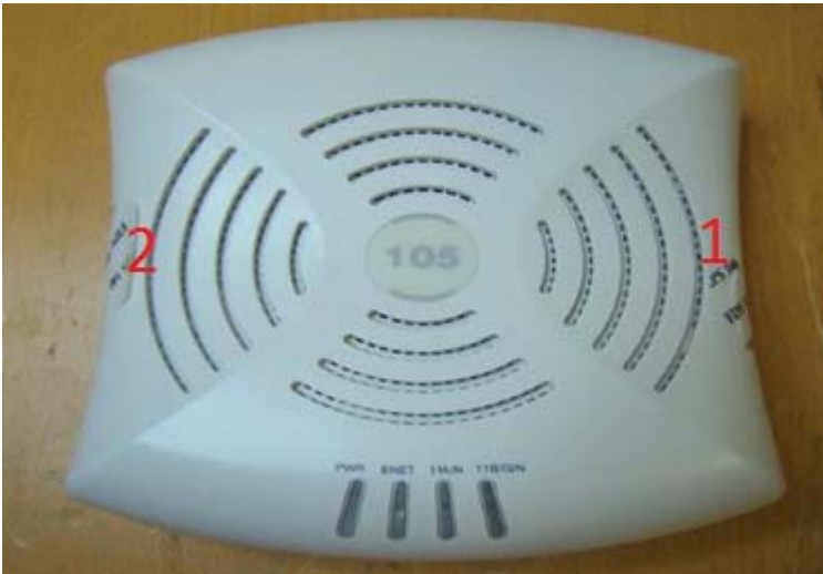
Figure 19 - Aruba AP-105 TEL placement top view
