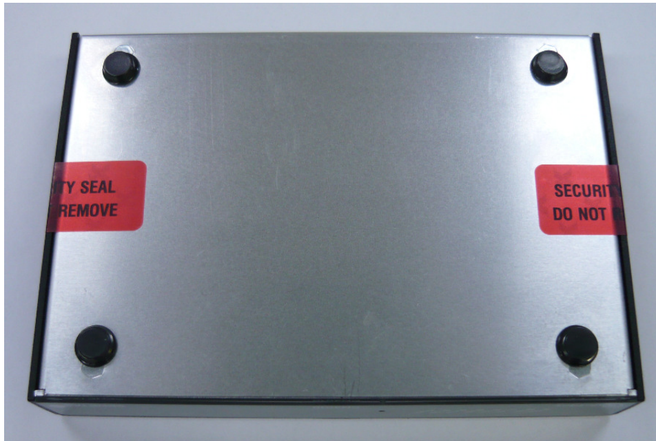
Figure 17 – CN4010 Factory installed tamper seals
