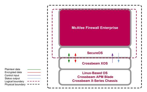
Figure 3 - MFE for Crossbeam Cryptographic Boundaries
