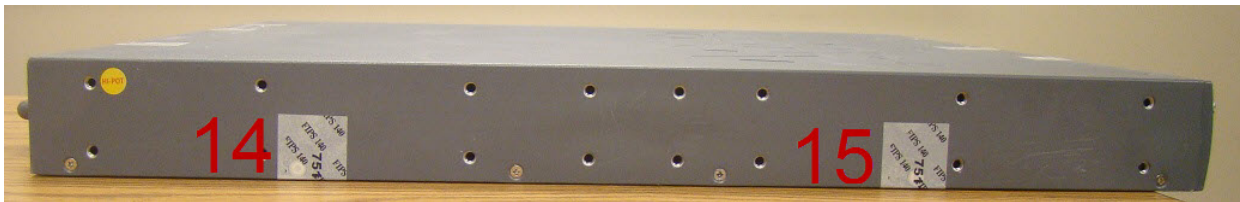
Figure 7 Required TELs for the Aruba 7200 Mobility Controller – Left Side
