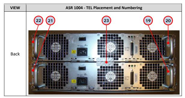
Figure 4. ASR 1004 TELs Installation
