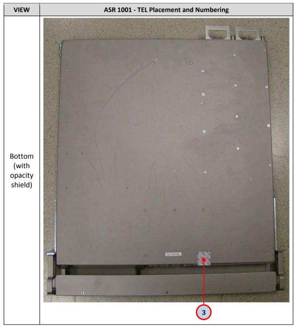
Figure 1. ASR 1001 TELs Installation
