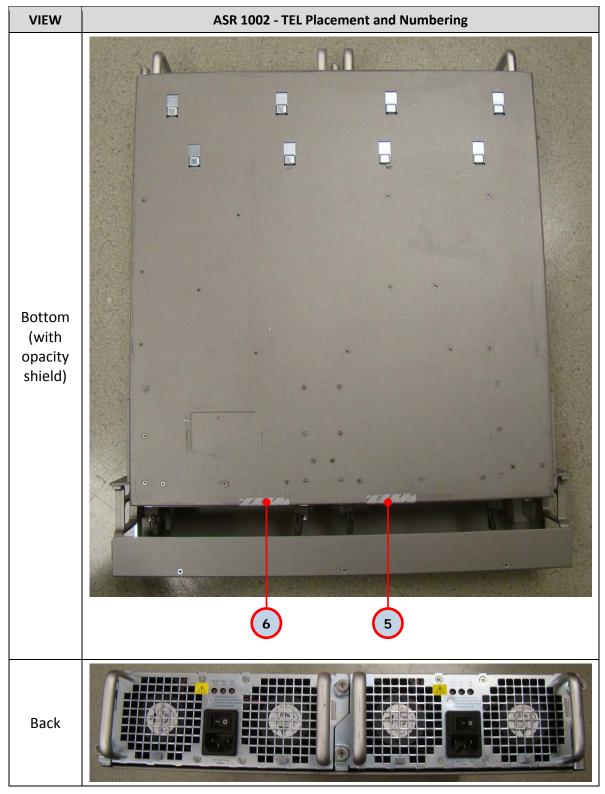
Figure 2. ASR 1002 TELs Installation
