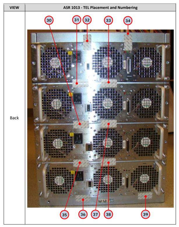
Figure 6. ASR 1013 TELs Installation
