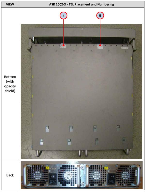
Figure 3. ASR1002X TELs Installation
