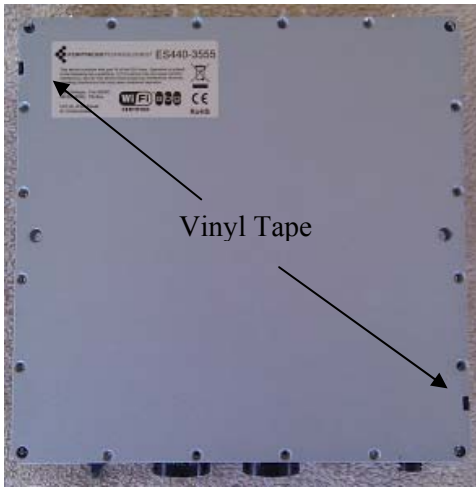
Figure 5: ES440 Tamper Evidence
