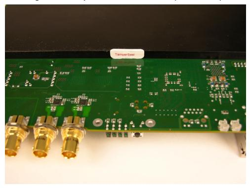
Figure 4 – Tamper Label Placement #2 (Bottomside)
