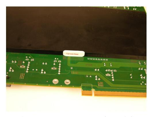
Figure 3 – Tamper Label Placement #1 (Bottomside)
