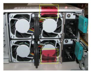
Figure 18 – Tamper-Evident Seal Application Positions (S5032/S6032 – Rear)
