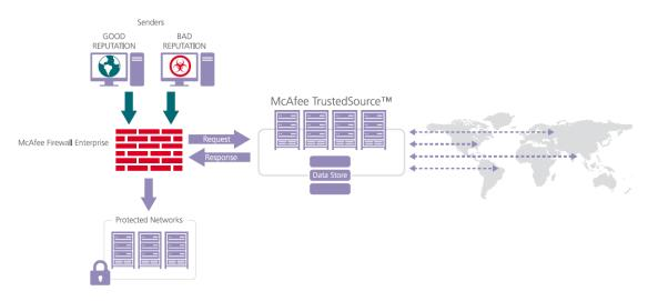
Figure 1 – Typical Deployment Scenario
