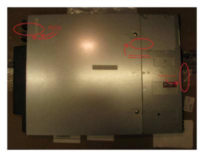
Figure 15 – Tamper-Evident Seal Application Positions (S4016)
