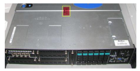
Figure 17 – Tamper-Evident Seal Application Position (S5032/S6032 – Top)
