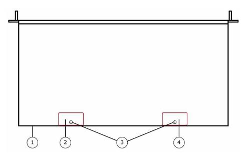
Figure 13 – Tamper-Evident Seal Application Positions (S1104)
