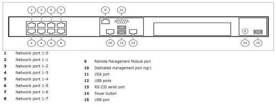
Figure 9 – Front Panel Features and Indicators for S3008
