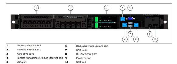
Figure 10 – Front Panel Features and Indicators for S4016
