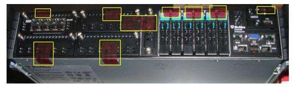
Figure 16 – Tamper-Evident Seal Application Positions (S5032/S6032 – Front)
