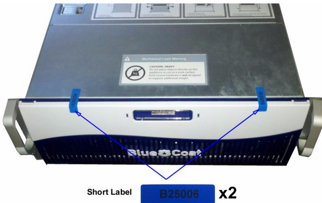
Figure 15 Front Bezel Label Application Points
