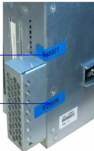
Figure 12 Tamper Evident Label Application – Small Louvered Shutter
