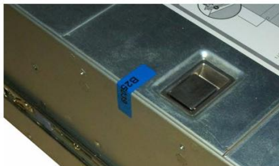
Figure 14 Tamper Evident Label Application – Top and Side of Appliance
