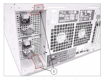
Figure 8 – Tamper-Evident Seal Application Positions (Power Supplies)
