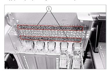
Figure 6 - Velcro Strip Placement in Rear of Chassis
