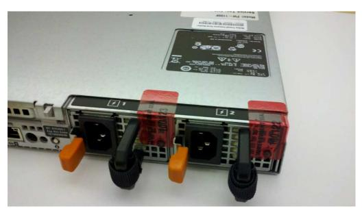
Figure 9 – Tamper-Evident Seal Application Positions (Power Supplies)
