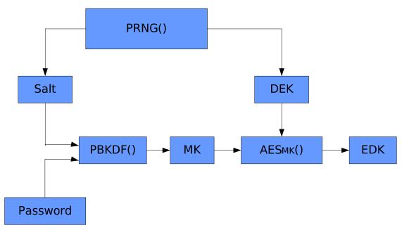
Figure 11: Overall Encryption Procedure
