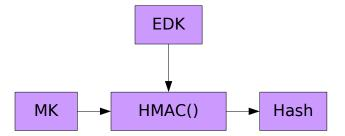
Figure 13: Message Digest Creation Using Master Key
