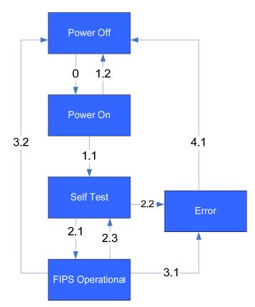
Figure 9: Crypto Module Finite State Machine
