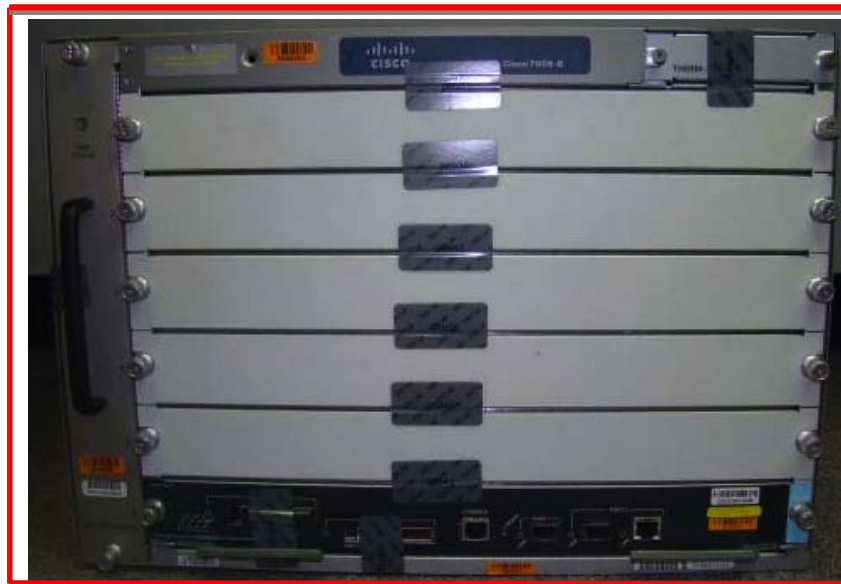
Figure 1 - Cisco 7606-S Router
