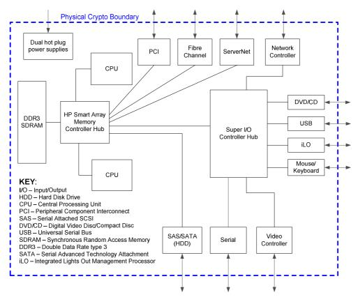
Figure 2 - Block Diagram of an HP ProLiant System
