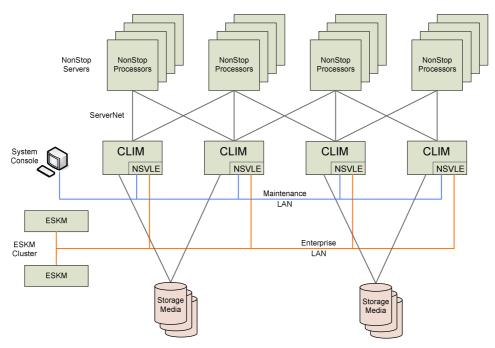
Figure I - Architecture of NSVLE Environment
