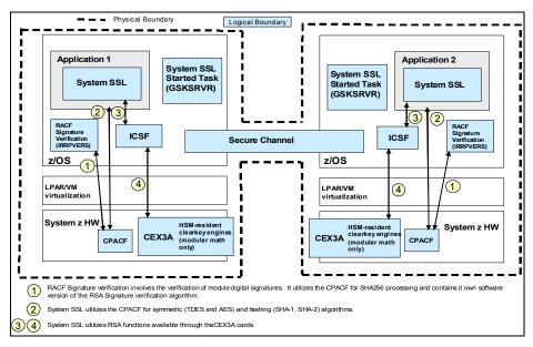
Figure 9 Validated Configuration with CPACF and CEX3A cards
