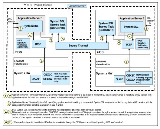
Figure 2 System SSL Cryptographic Module in a z/OS Sysplex Environment
