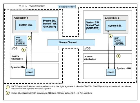
Figure 7 Validated Configuration with CPACF only
