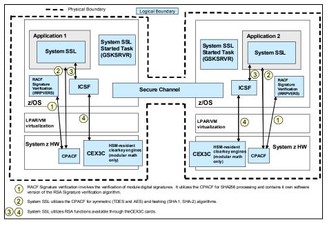
Figure 8 Validated Configuration with CPACF and CEX3C cards
