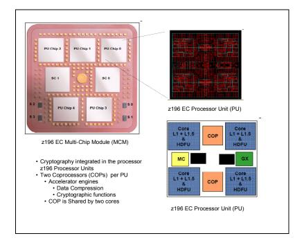
Figure 6 Processor Unit MCM with CPACF COP chips
