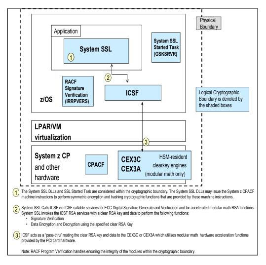
Figure 1 System SSL Cryptographic Module
