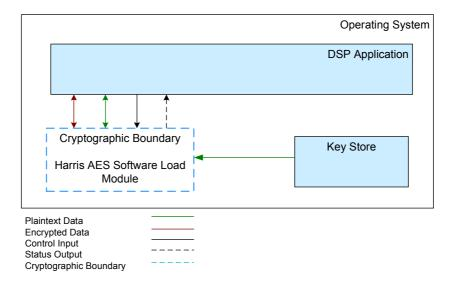
Figure 3 - Logical Cryptographic Boundary
