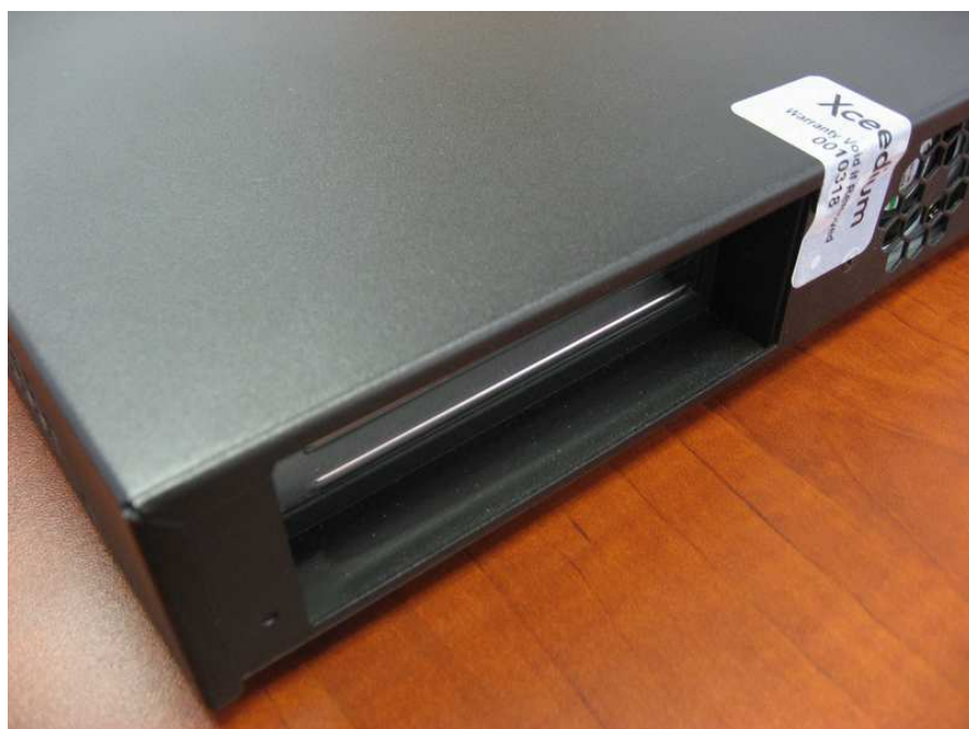
Figure 2 – Tamper Evidence Label Placement
