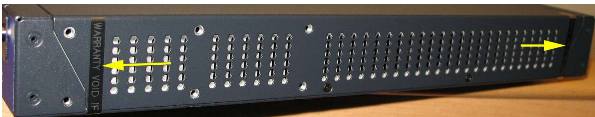
Figure 5. SRX240 Tamper Evident Seal Location (Right Side)
