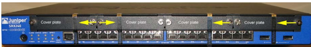
Figure 4. SRX240 Tamper Evident Seal Location (Front)
