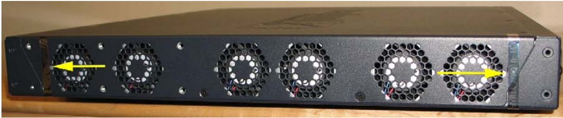
Figure 6. SRX240 Tamper Evident Seal Location (Left Side)
