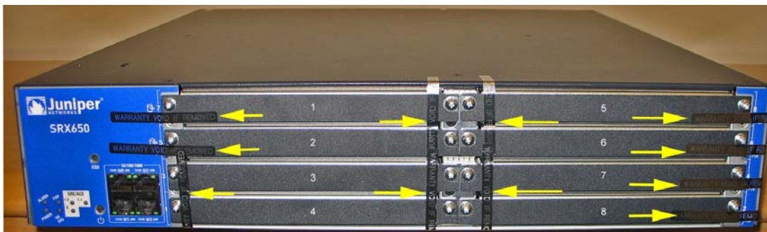
Figure 7. SRX650 Tamper Evident Seal Locations (Front)
