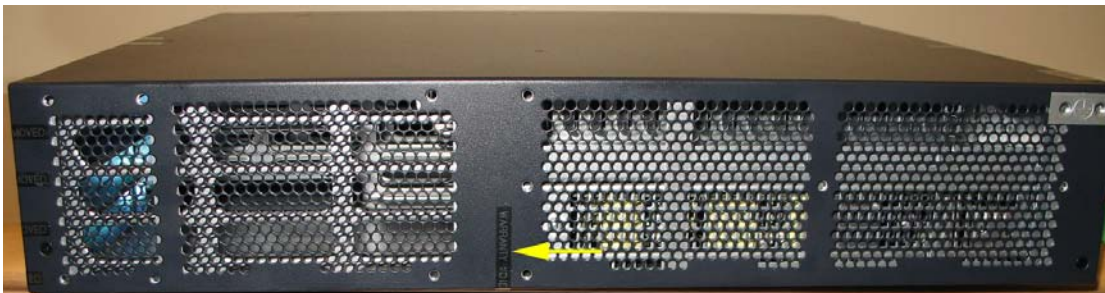
Figure 9. SRX650 Tamper Evident Seal Location (Right Side)
