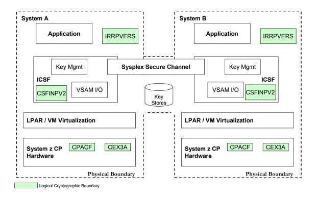
Figure 8 Validated Configuration with CPACF and CEX3A.
