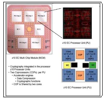
Figure 6 Processor Unit MCM with CPACF COP chips
