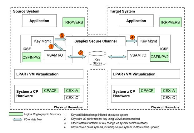
Figure 2: ICSF PKCS #11 Cryptographic Module in a z/OS Sysplex Environment
