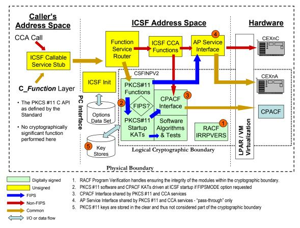
Figure 1: ICSF PKCS #11 Cryptographic Module
