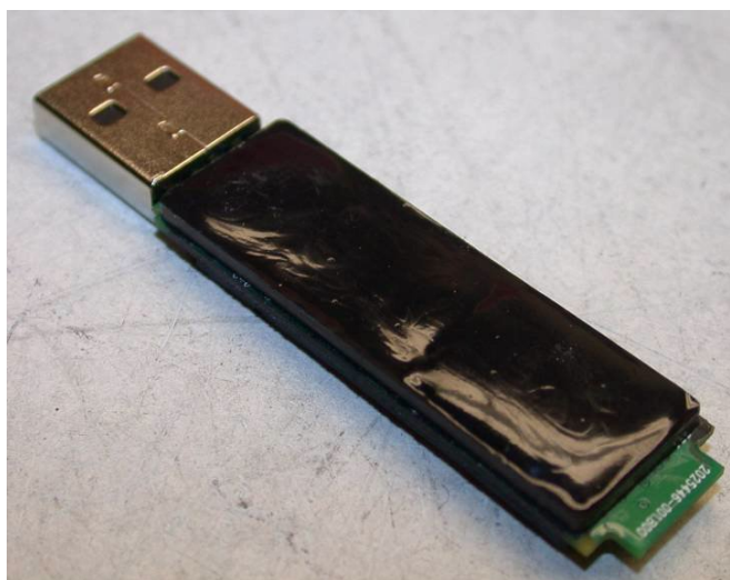
Figure 2 Hydra PC FIPS Sector-based Encryption Module (Underside)
