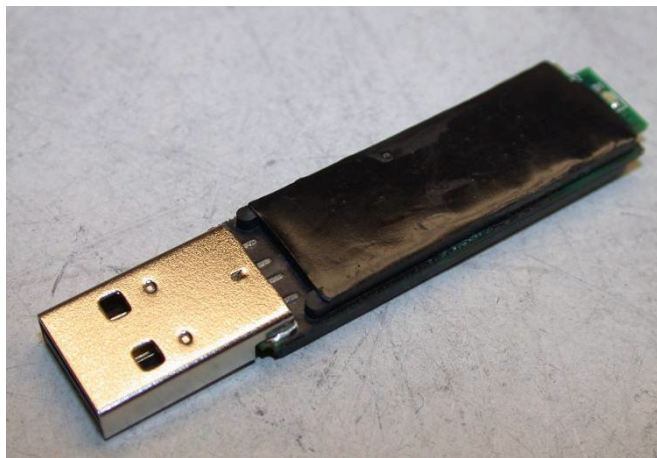
Figure 1 Hydra PC FIPS Sector-based Encryption Module (Topside)
