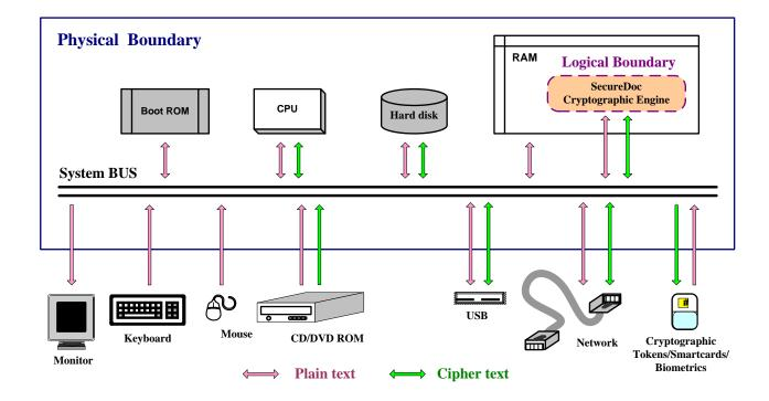
Figure 1 - Cryptographic Module Block-Diagram
