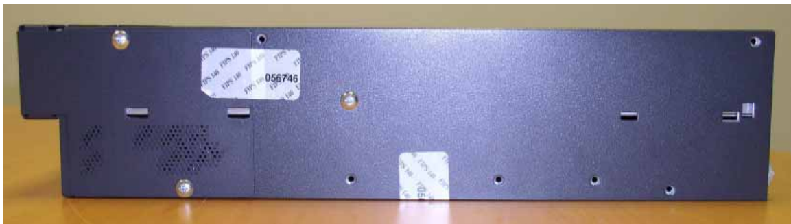
Figure 5 Placement of Tamper evident labels over the opacity shield and the removable cover
