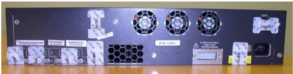
Figure 4 Placement of Tamper evident labels over the serial port, service port, and stack ports
