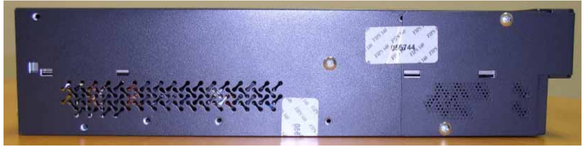
Figure 6 Placement of Tamper evident labels over the opacity shield and the removable cover
