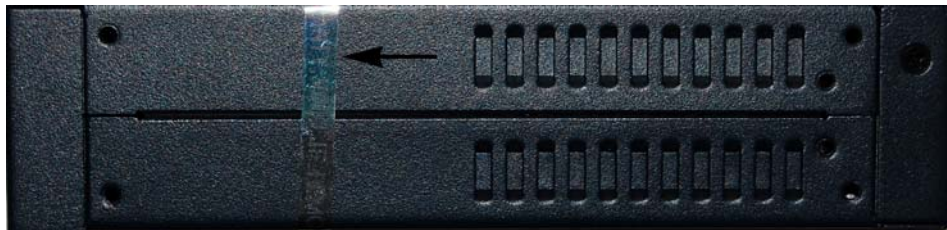
Figure 7: Side of both SSG 5 and SSG 20 devices, with location of tamper evident seal
