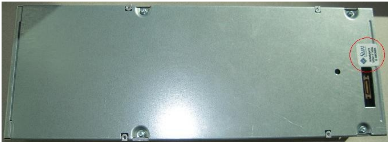
Figure 10: Tamper Evident Seal on Bottom
