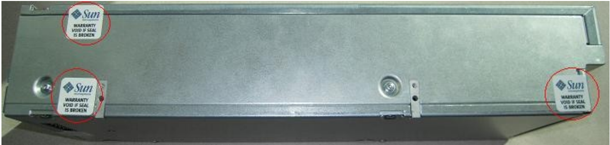
Figure 9: Tamper Evident Seals on Right Side
