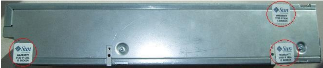
Figure 8: Tamper Evident Seals on Left Side
