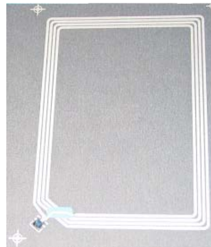
Figure 3: Module embedded in the cover of an e-Passport
