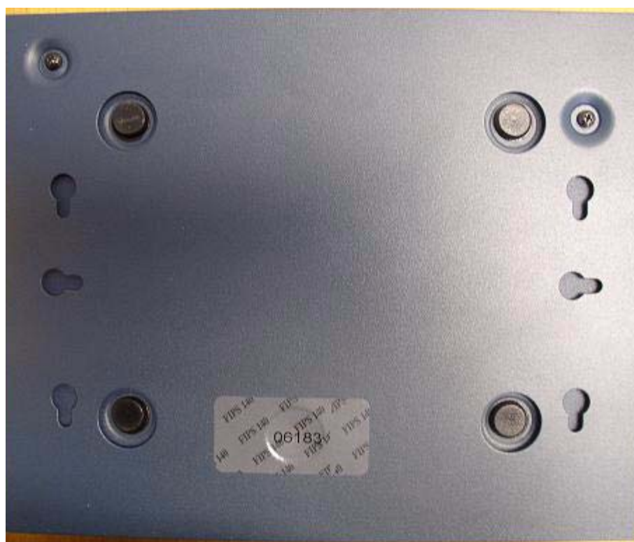
Rack-Mountable Enclosure with Tamper Evidence Label Placement
